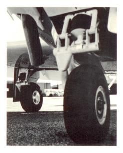
Rugged Mooney gear has no fancy hydraulics or oleos to run up shop bills. Positive-action energy-absorbing electric gear retracts in three seconds, extends in two.
